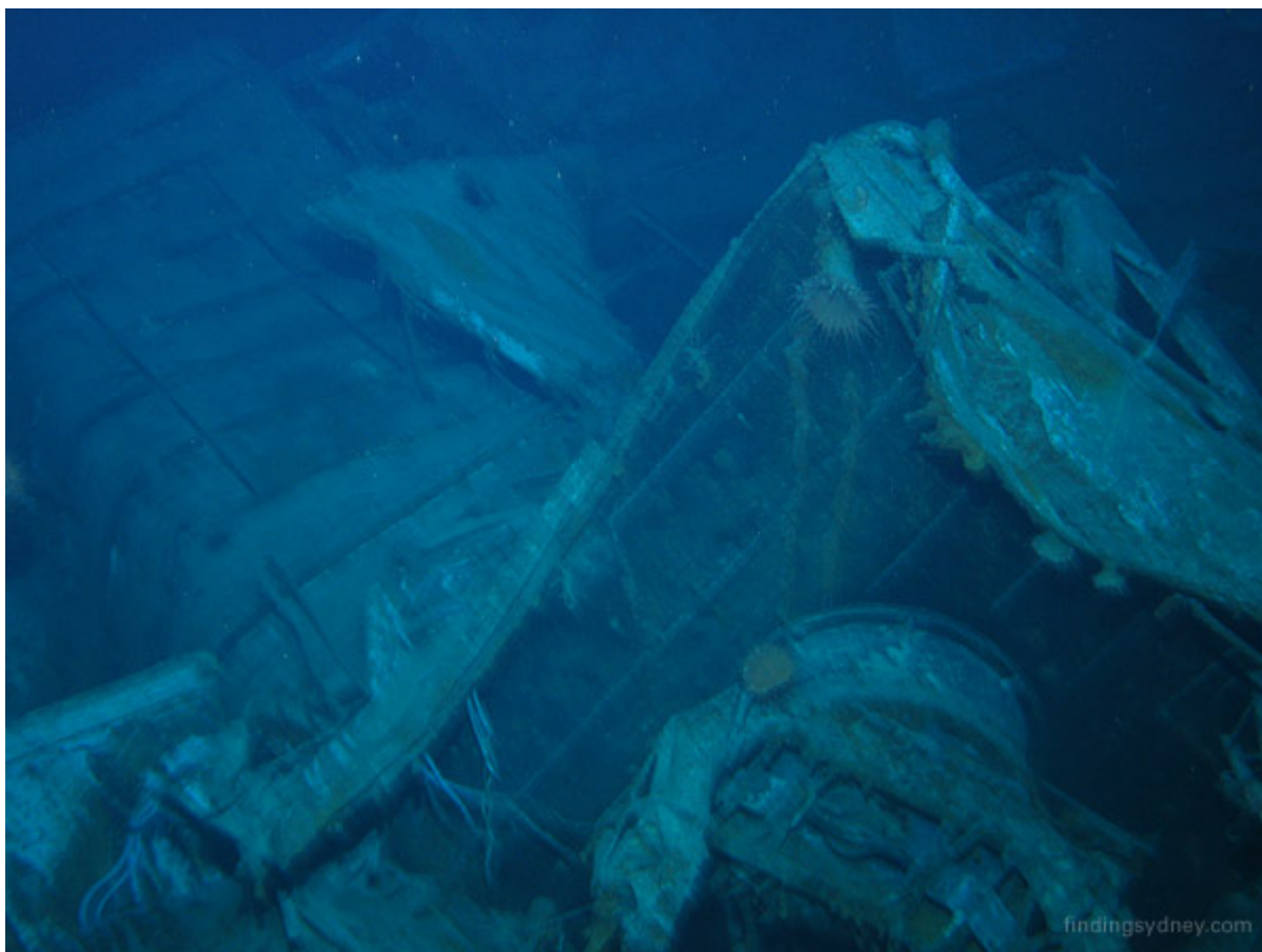
Above Photograph: Upturned searchlight platform torn away from forward funnel.
