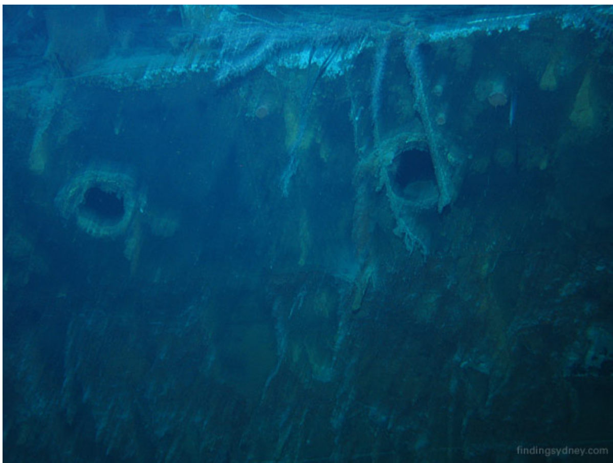
Above Photograph: Upturned searchlight platform torn away from forward funnel.
